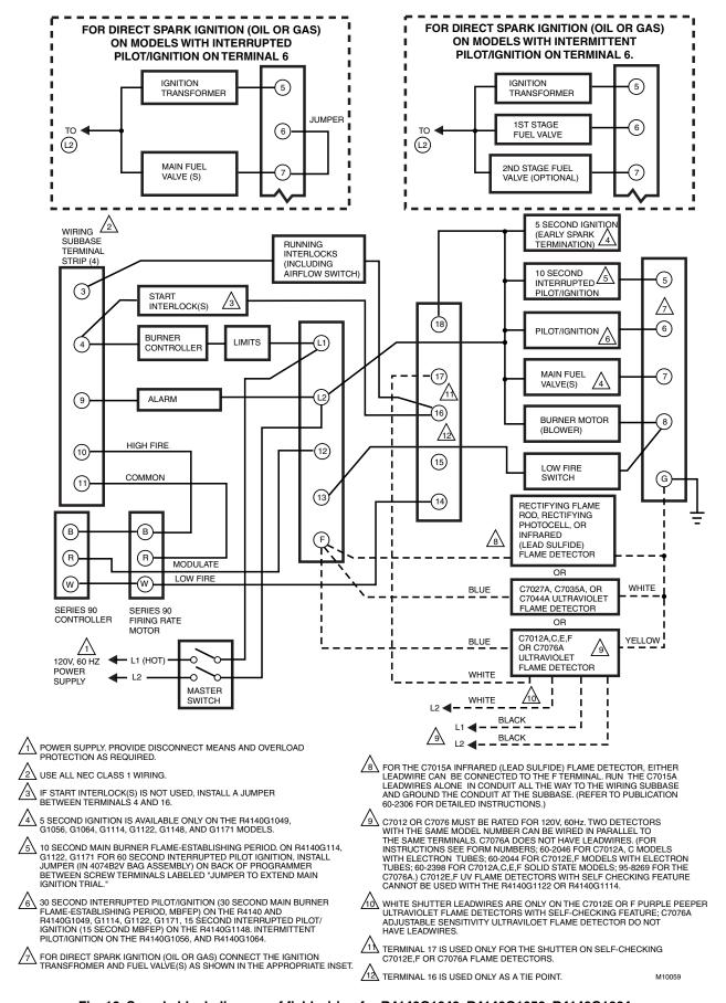
Fig. 16. Sample block diagram of field wiring for R4140G1049, R4140G1056, R4140G1064, R4140G1114, R4140G1122, R4140G1148 and R4140G1171 Programmers.
